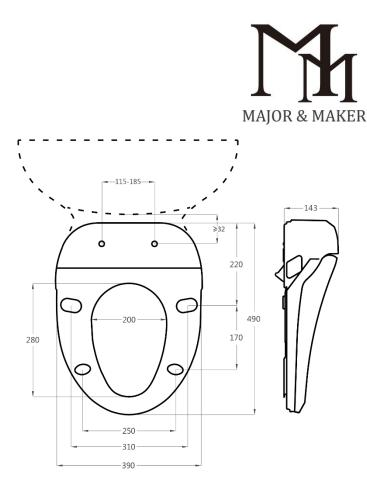
Overall product dimensions: **490 x 390 x 143 mm** Seat opening dimensions: **280 x 200 mm** Weight: **5.1 kg** Type of control: **Remote control + Simplified side panel**
